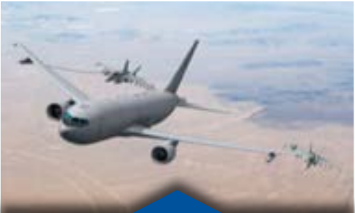
The Boeing KC-46A Tanker demonstrates its ability to simultaneously refuel two F/A-18 Super Hornet aircraft from wing air refueling pods (Boeing photo illustration).
